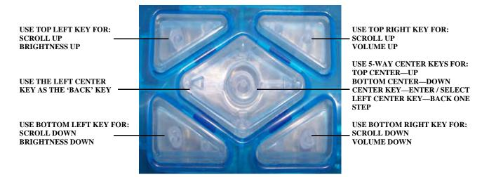
The iLightz has 9 total keys: 4 are on the outer perimeter and the center is a 5-way keypad.
