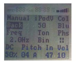
To move from one value to the next, use center keys or Manual / Back. To change any of the following particular values, use right side keys on keypad (Top right = increase, bottom right = decrease)
